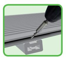
After placing the end clip to each joist as to the middle of the joist, perforate with suitable drill at 45° angle Screw
