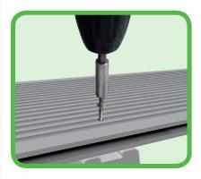
Once you have fitted the final board, drill the Deck in the middle part of each joists using a drill with a bit suitable for 90° angle, then screw the hole you have drilled.
